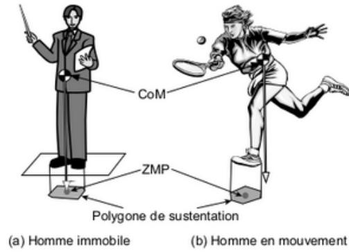
Figure 3.3 – CoM, ZMP et polygone de sustentation.
