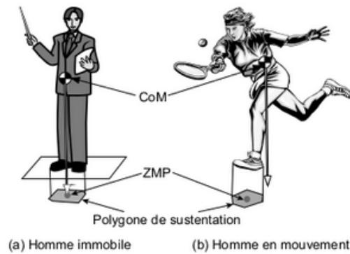
Figure 3.3 – CoM, ZMP et polygone de sustentation.
